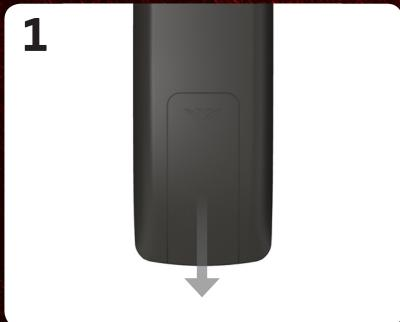
Remove the battery cover by pressing gently and sliding away from the remote.
